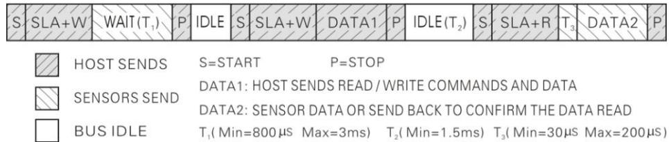
**Figure 13:** I<sup>2</sup>C Sensor reading and writing a complete sample chart
