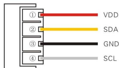
Figure 1: AM2315wiring diagram
