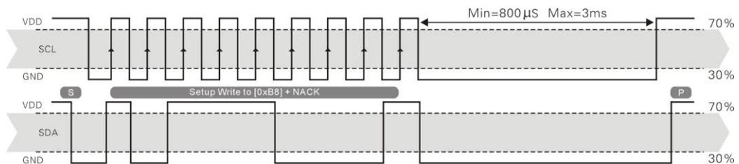
**Figure 14:** Wake-up sensor
