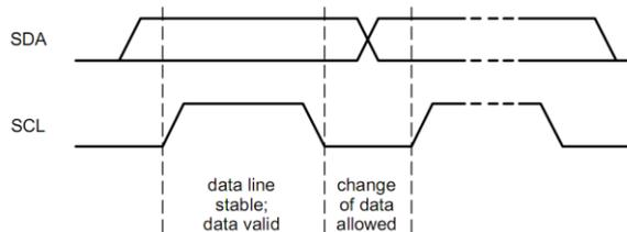
Figure 5: I<sup>2</sup>C Bus bit transmission
