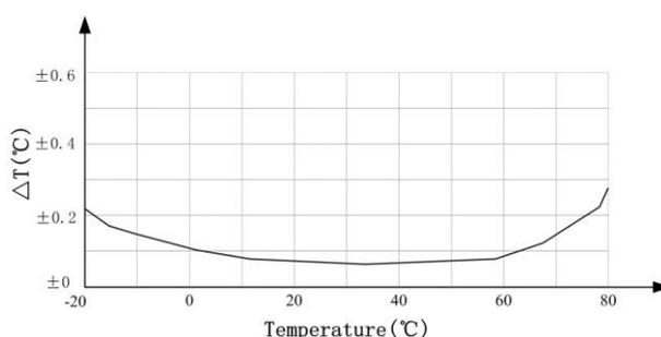
Figure 3: The maximum temperature error of temperature sensor
