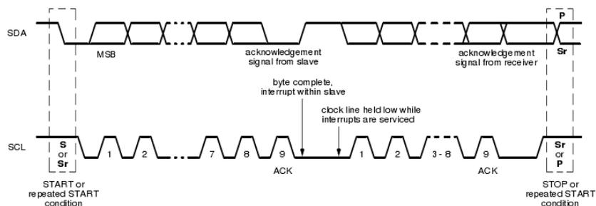
Figure 7: I<sup>2</sup>C Bus data transfer
