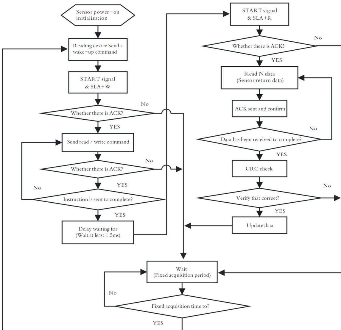
Figure 17: Sensor with I2C read flow chart
