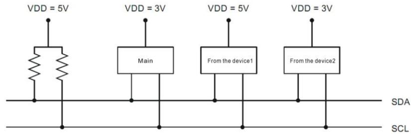
Figure 4: I<sup>2</sup>C typical configuration
